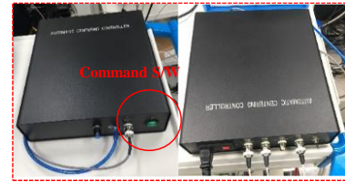
Fig. 4 Manufactured control box for the impact actuator
