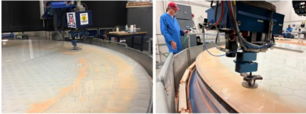
Fig. 3 GMT Segment 3 being polished with a 40 cm pitch lap at left and a 10 cm lap at right. Both laps are driven by the same orbital polisher [25].
